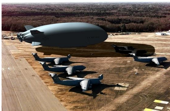
An artist's impression of the scale of how a hybrid air vehicle with a 200-ton payload capacity would appear alongside other aircraft, below.
